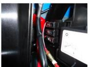
Attention: Do not use fuses that are out of specification compared to the original fuse. Any fuse installed that is not to specification can seriously damage the electrical system.
