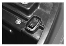
Attention: Do not change the switch's position while the engine is still running. Change position only when the vehicle is parked.
